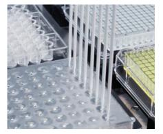
Cap piercing using washable fixed tips with the liquid displacement Flexible Channel Arm
