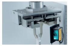
Tube handling with the Robotic Gripper Arm
