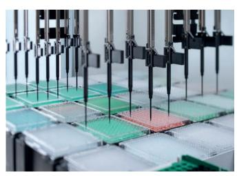
Up to 16 separate pipetting channels can be used to enhance throughput for applications such as hit-picking
